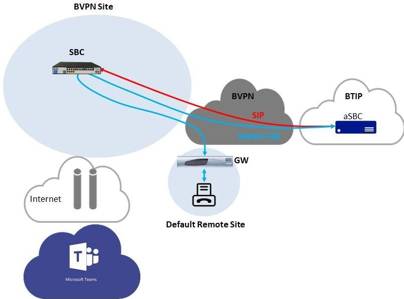
In this architecture FAX device is connected to an analog telephony adapter. It is integrated with DR SBC which can be placed in other remote site or in datacenter. DR SBC with no directly connected endpoints can be virtualized.
