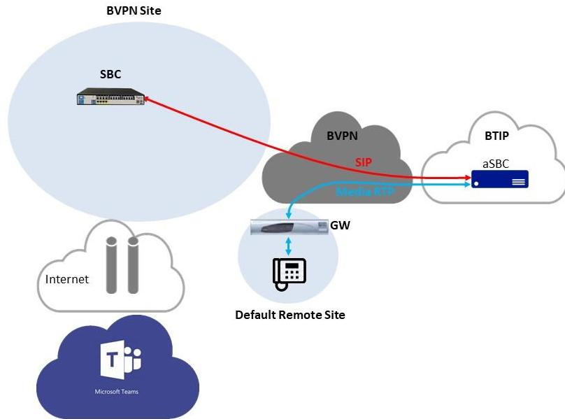
In this architecture, device is connected to an analog telephony adapter. It is integrated with DR SBC which can be placed in other remote site or in datacenter. DR SBC with no directly connected endpoints can be virtualized. Note that direct media with BTIP/BTalk has been validated in this case.
