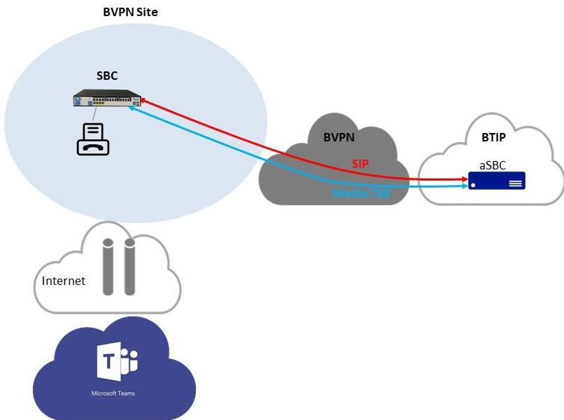
The analog FAX device can be connected directly to hardware DR SBC with FXS ports. Call is routed directly between Business Talk / Business Talk IP and FAX.
