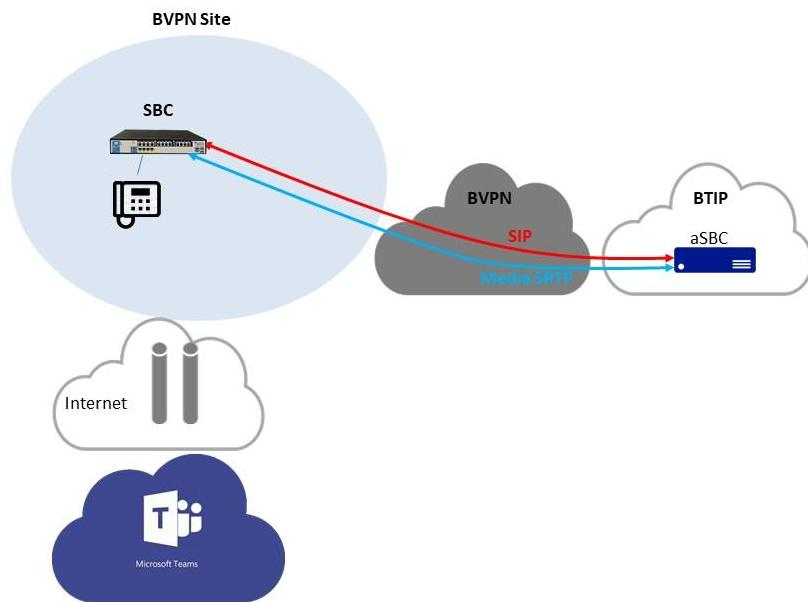
The analog phone can be connected directly to hardware DR SBC with FXS ports. Call is routed directly between Business Talk / Business Talk IP and analog device.
